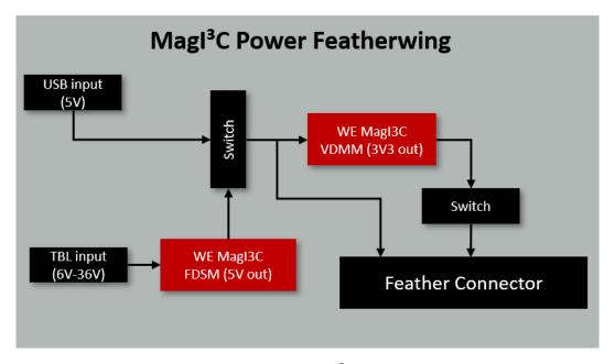
Figure 2: Block diagram - MagI<sup>3</sup>C Power FeatherWing
